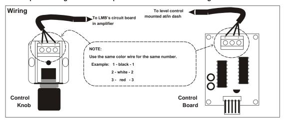
Installation of Large Mouth Bass™ circuit board and level control
