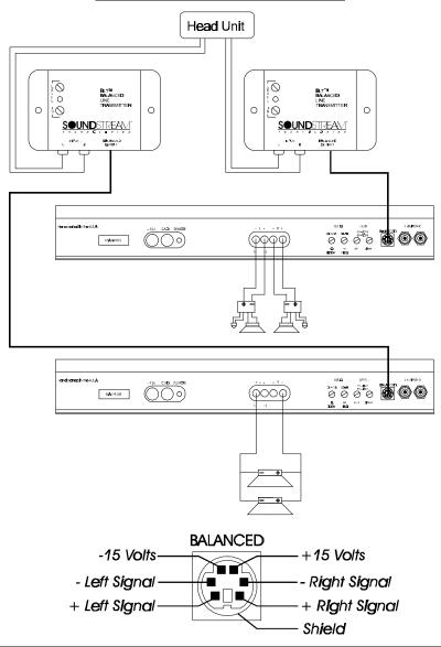
NOTE: The pin configuration shown in the diagram is the view looking into the Balanced input jack on the amplifier and the  $BLT^{TM}$ .
